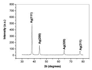
**Figure 2.** XRD spectrum of the hierarchical bowl-like structures synthesized after heated at 360 °C for 3 h using AgAC as precursor and the colloidal monolayer as a template.
