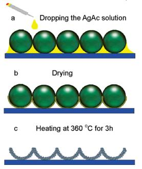
was used as the electrolyte and the pH was kept to 5.0. PS colloidal monolayer was heated at 120 °C for 30 min in order to tightly adhere to the conduct substrate. The deposition voltage was controlled to 1.5 V, and the deposition time was 30 min. After electrodeposition, the PS colloidal monolayer was removed by ultrasonically washing in CH<sub>2</sub>Cl<sub>2</sub> solution, and silver pore arrays film was finally prepared.
