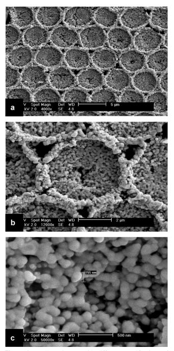
**Figure 1.** FE-SEM images with different magnifications of hierarchical bowl-like array film. (a) A typical FE-SEM image of hierarchical bowl-like array film obtained using the PS colloidal monolayer with sphere size of the 5  $\mu$ m. (b) An image of a feature bowl-like unit. (c) An image of bowl bottom with larger magnification.
