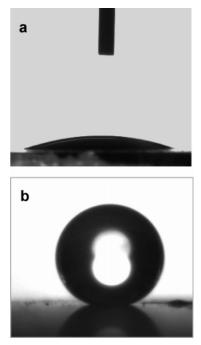
**Figure 4.** Water droplet shapes of hierarchical bowl-like structured film: (a) before chemical modification with thiol, CA: 23°, (b) after modification, CA: 169°.
