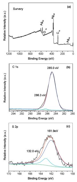
**Figure 5.** XPS spectra of the hierarchical structures after chemical modification with 1-hexadecanethiol. (a) XPS survey spectrum. Panels b and c are C 1s and S 2p core level, respectively.
